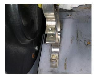
It was reported that a technician found a cracked oil cooler blower bearing support bracket. He was having trouble aligning the blower short shaft. This support bracket was replaced by a 4129104-19 bracket which has a thicker bottom flange. Enstrom recommends occasional cleaning of the fan squirrel cage fan to prevent out of balance, and installation of the -19 support bracket.
