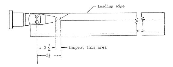
Should a crack be found, the blade must be retired from service, and we request that the Enstrom Corporation be advised of the defect.
