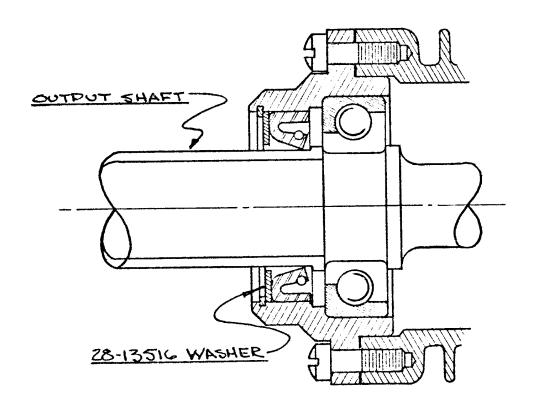
To install the 28-13516 washer, remove the tail rotor assembly and pitch link retainer assembly. Remove Truarc seal retainer, install washer 28-13516by pressing output shaft seal inward .050 of an inch. Reinstall Truarc and reassemble.
