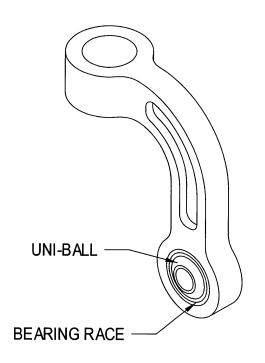
Figure 2. Uni-Ball Bearing Location
