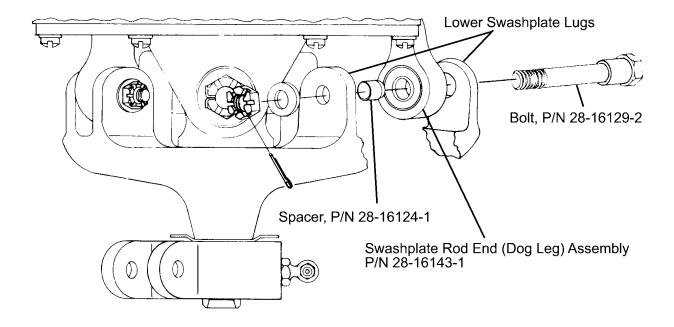
Figure 1. Swashplate Rod End (Dog Leg) Assembly Location
