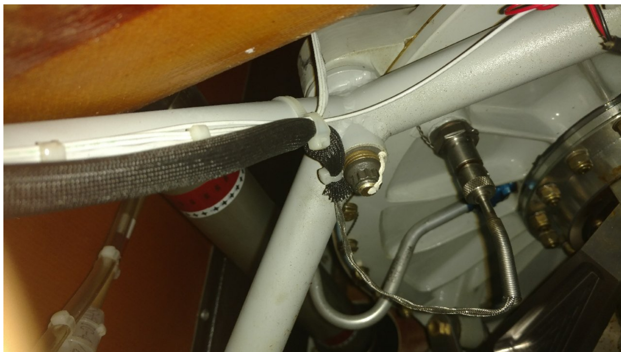
Figure 1. Photograph of Forward Left Mount with Transmission Installed (Photo taken through engine access door)
