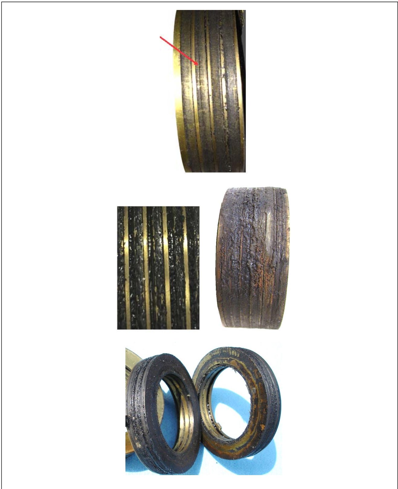
Figure 1. Early stage of delamination (top, at the arrow tip), rubber extrusion (middle, left and right), and rubber extrusion with shear (bottom)
