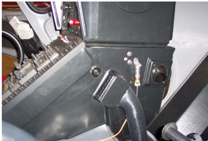
Figure 3. Velocimeter installed on the lower instrument panel.
