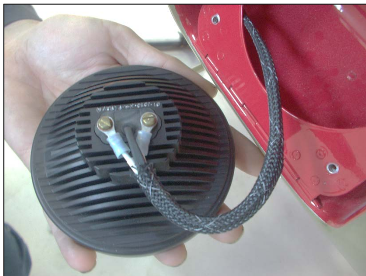
Figure 4. Wire bundle with sleeving (Rev. A shown)
